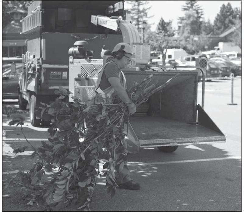
Wear all the required PPE when working with a chipper or shredder.
